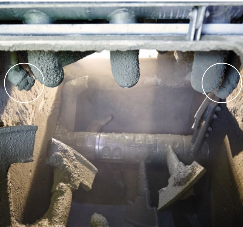
twin-shaft mixer before and after cleaning
