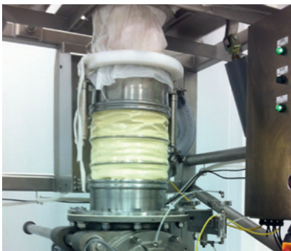
Bigbag station – outlet
