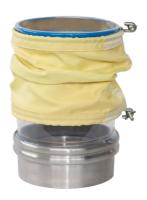
The Kevlar cover is attached to the outside of the BFM® spigot with butterfly screws — hence tool free — and can be removed easily at any time to check or replace the BFM® fitting underneath.
