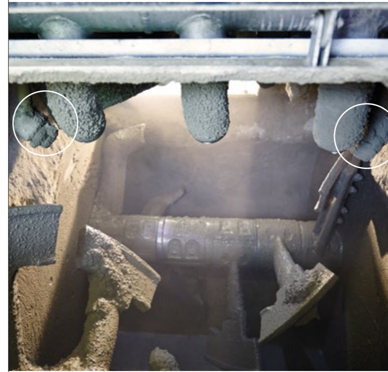
twin-shaft mixer before and after cleaning
