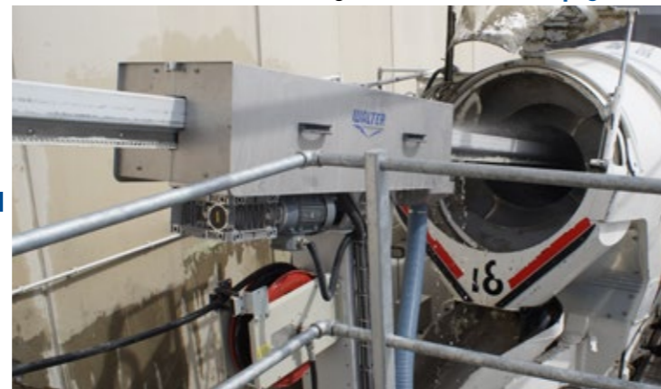
>> Inside cleaning for truck mixer drums page 10-11
